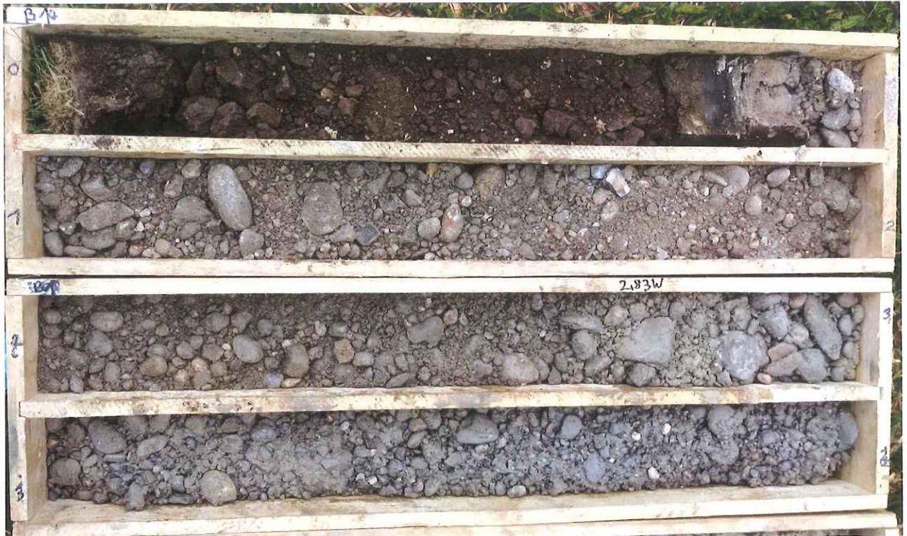
**Bohrkern B 1 4,0 - 8,0 m:**
